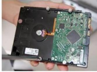
2. Attach four screws in the HDD (Turn just three times).
