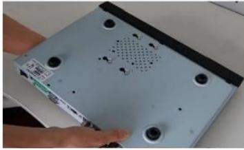
4. Turn the device upside down and then turn the screws in firmly.
