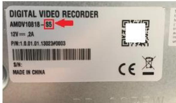
For example, if the model number for the device has a AMDVXXXXX-S3 or above end notation the below initialization procedures pertain to that device. For more information on the initialization process of these model DVRs, refer to the instruction set provided below.
